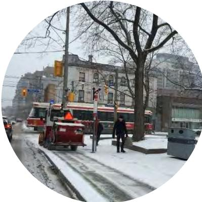
Sidewalk plow clearing a vertically separated cycle track
