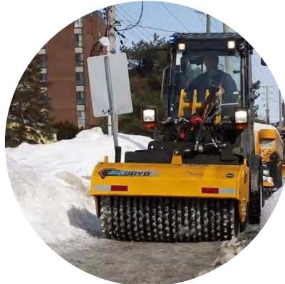
Blue gryb rotating icebreaker crushing ice on a sidewalk
