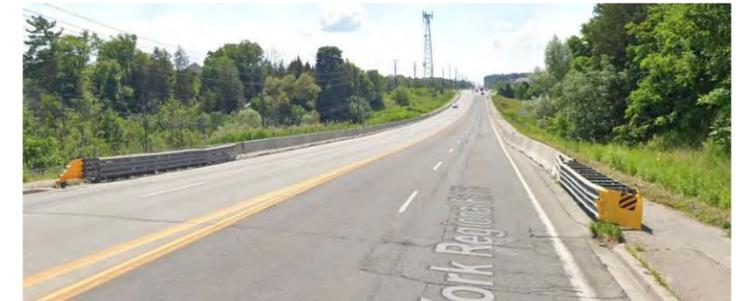
Figure 12 - Example of barrier protection of paved shoulder on Rutherford Road in Vaughan
