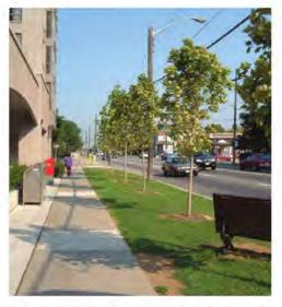
Figure 4.4 Offsetting tree planting from wires can help mitigate the visual impacts of overhead wiring.
