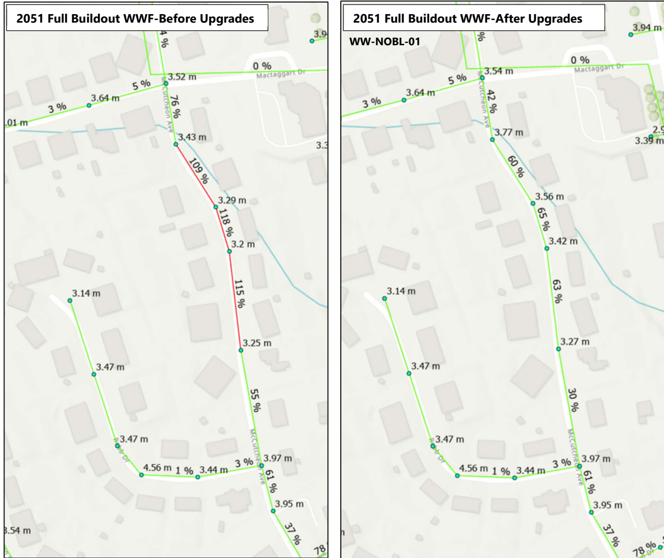
Figure 3: Nobleton Simulated Pipe Capacity% and Manhole Freeboard under WWF Before and After Upgrades
