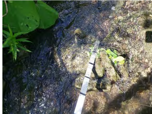
Riffle sequence downstream of the crossing. Riffle substrate consisted of sand, gravel, and cobble.
