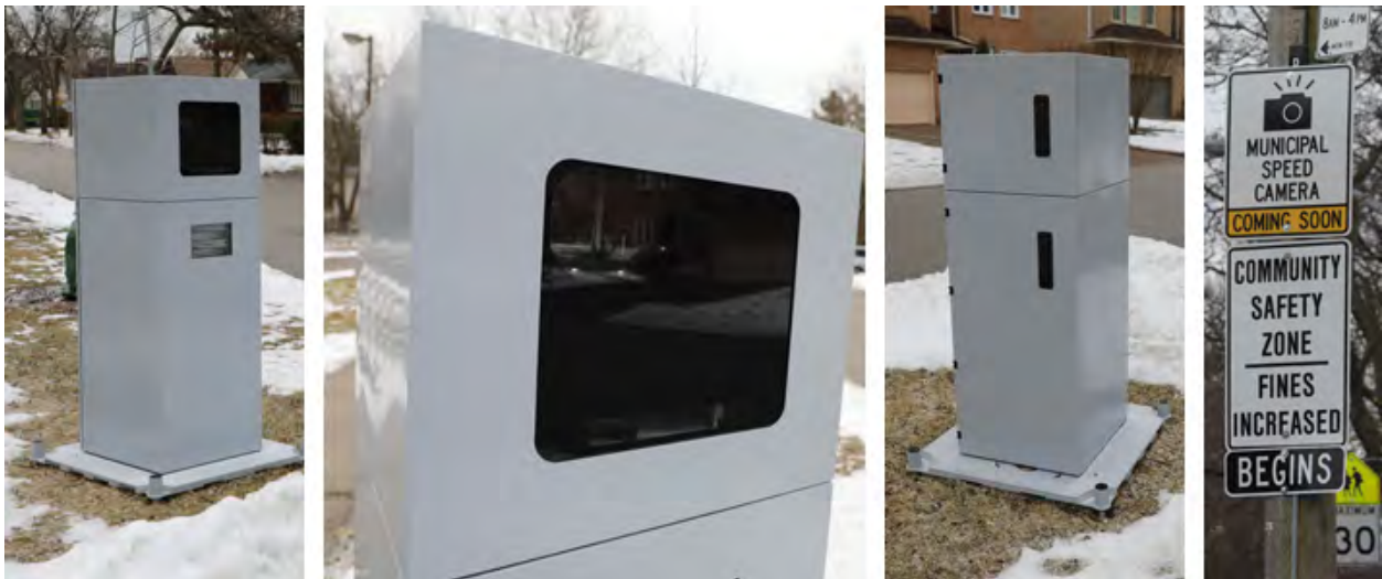
Figure 3-7: Automated Speed Enforcement Device and Corresponding Signage
